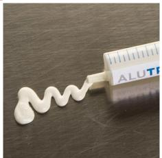
Thermal compound to increase heat conductivity between heat sink and electrical package by filling up pockets of air between interface contacts. For an area of 100x100 mm (unmilled extruded profile) about 4,0g of thermal compound should be spread out as a thin film.
