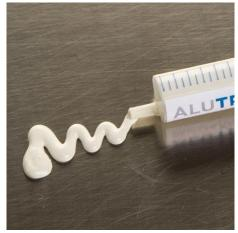
Thermal compound to increase heat conductivity between heat sink and electrical package by filling up pockets of air between interface contacts. For an area of 100x100 mm (unmilled extruded profile) about 4,0g of thermal compound should be spread out as a thin film.
