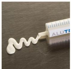
Thermal compound to increase heat conductivity between heat sink and electrical package by filling up pockets of air between interface contacts.
