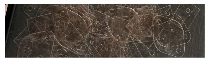
Mica panels are used in conjunction with insulating bushings for insulated assembly of semiconductors, e.g. on heat sinks.
